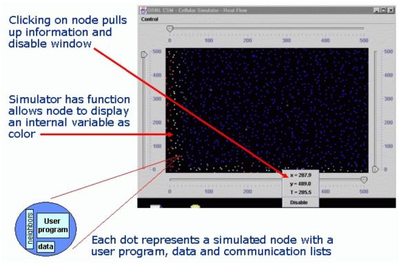
Figure 2. User interface to the ORNL 100,000 processor simulator.
