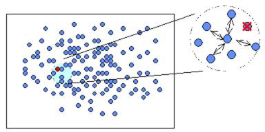
Figure 1. Meshless formulation of 2-D finite difference application using a uniform distribution of nodes and a user selected number of local neighbors.
